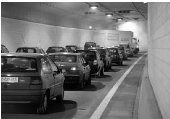
Figure 2. One of the nine tests that were made in the Benelux tunnel in the Netherlands to collect data on road tunnel evacuation.
